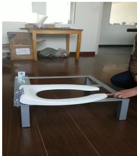
时钟12点至15点先快后慢再快的三段动作效果产品 Three speeds of motion from 12 to 15 o'clock direction.
