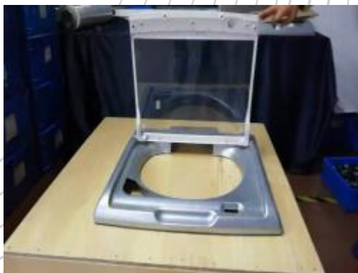
匀速闭合最后角度加快效果的视频展示 Video of closing in uniform speed first and then fast.
