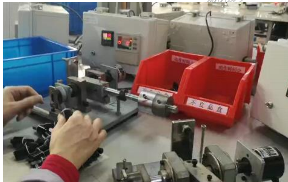
视频为缓冲器生产工序中全检方式 This is how we full inspect the product during production
